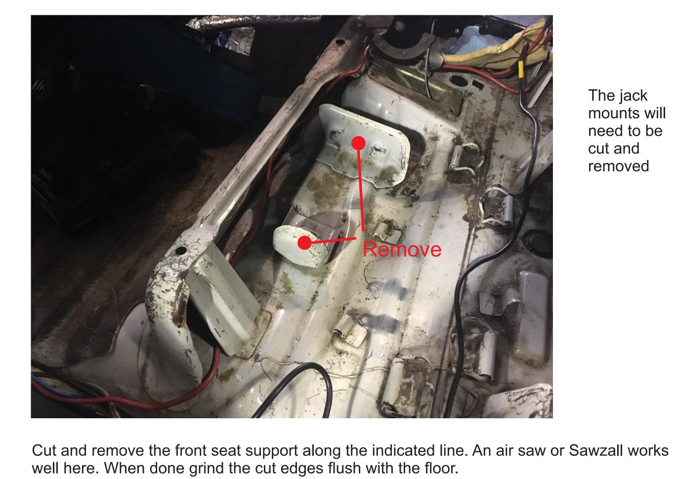
The jack mounts will need to be cut and removed
