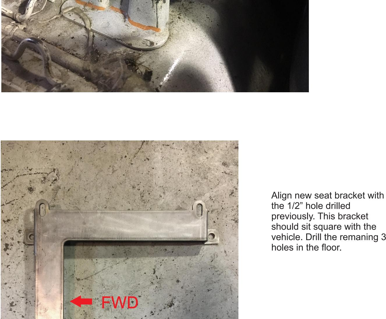
previously. This bracket should sit square with the vehicle. Drill the remaning 3 holes in the floor.
